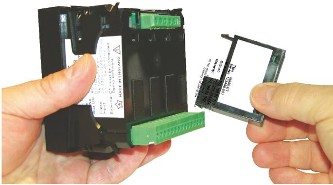
The Ethernet pod (option) can be installed into either position in the back of a M850 power meter. The pod incorporates a 10/100Base-T Ethernet controller. The protocols supported are:
