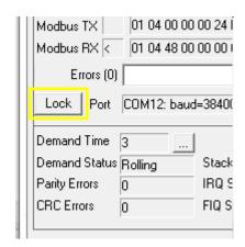
It's worthwhile noting the address of a device and, if it's locked, all the network settings (address, baud rate, stop bits and parity).
